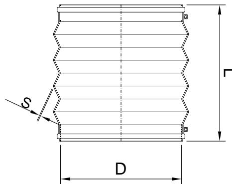
TPE flexible connector with steel bands
