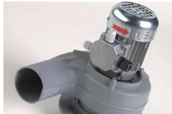
Small centrifugal fans of Frv type for conveying aggressive and explosive gases, steams and vapours with dust content < 5 mg/m<sup>3</sup> and max. temperature 40°C, ambient temperature max. 40°C.
