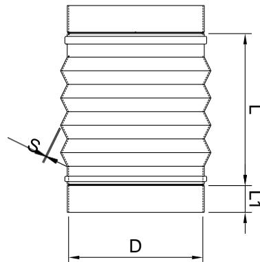
PVC flexible connector with sockets
