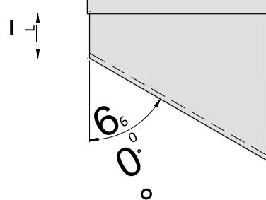
The air intake vent is made with a spigot end as a standard. It can also appear as a socket (see figure) or flanged version. The minimum length L is 100 mm. Standard width of the socket - 60 mm
