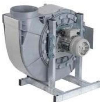
Centrifugal fans of **FRv** type for conveying aggressive and explosive gases, steams and vapours with dust content < 5 mg/m<sup>3</sup> and max. temperature 40°C, ambient temperature max. 40°C.
