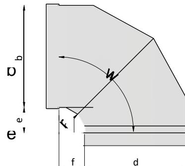
Standard chemically resistant sectional arcs are made with angles: 15°, 30°, 45°, 60°, 75° and 90°, both ends with connection sockets. They can also appear in other configurations – depending on needs- (socket **M** - flange **K** - spigot **B**).
