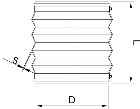
PVC flexible connector with steel bands
