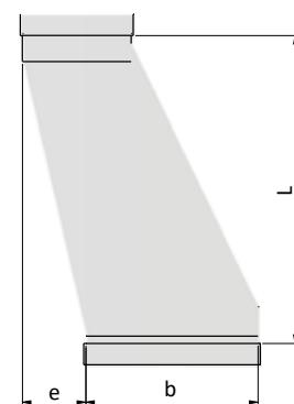
The asymmetric reduction has both ends ended in connection sockets as standard.
