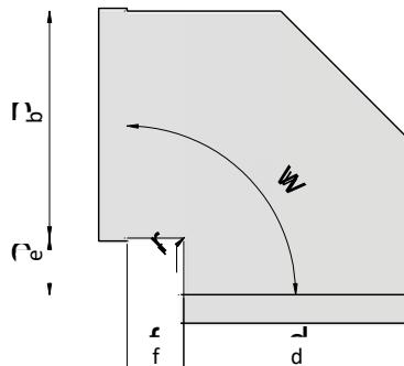
Ventilation elbows are standardly made with angles: 15°, 30°, 45°, 60°, 75° and 90°, both ends are ended with sockets. They can also be available in other configurations, as required (socket **M** - flange **K** - spigot **B**).
