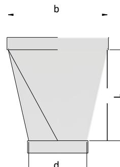
The transition from rectangular to round section has both ends ended with connection sockets.
