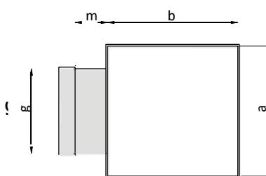
Tees are normally produced with exits of 90° and 45°. They can be used as a reduction or equal flow ones, with all ends ended by connection sockets as standard.
