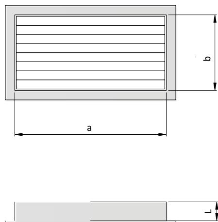
Intake/exhaust grid can be equipped with either permanent diagonal blinds or with the net of perforated panel. Connection ferrules from the duct side as spigot ones **B**. Wall thicknesses depending on medium parameters as well as duct size (axb).
