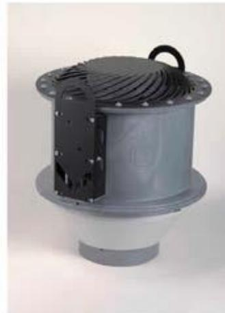
Roof fans of **FDvF** type for conveying aggressive and explosive gases, steams and vapours with dust content < 5 mg/m<sup>3</sup> and max. temperature of 40°C, ambient temperature max. 40°C.
