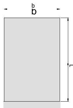
Standard ventilation ducts are made in the following lengths: 1000, 1500, 2000 and 3000 mm, both ends are spigot. Duct ends may also be available in other configurations, as required (socket **M** - flange **K** - spigot **B**). Wall thicknesses and possible ribbing depending on medium parameters. Standard width of the socket - 60 mm
