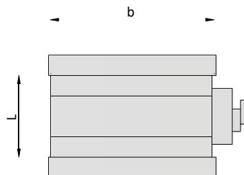
The throttle can be made as single- or multi-plane. Connection ferrules as socket **M**, flanged **K** or spigot **B** ones. The equipment is controlled manually as a standard, but depending on requirements it can be adapted to electric or pneumatic drives. Wall thicknesses and possible ribbing depending on medium parameters as well as duct size (axb). There is a possibility to produce the throttles with grid.
