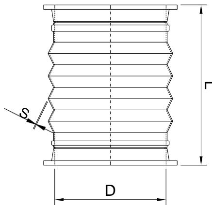
PVC flexible connector with flanges
