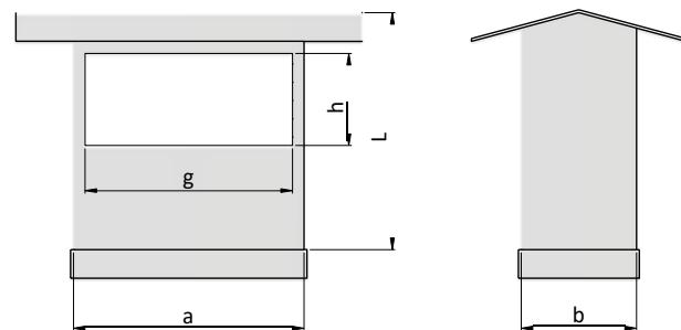
Air intake vent/roof exhaust is equipped with diagonal blinds or perforated panel. Connection ferrules as socket **M**, flanged **K** or spigot **B** ones. Wall thicknesses and possible ribbing depending on medium parameters as well as duct size (axb).
