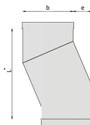
Both ends of plinth are ended with connection sockets as a standard. It can also be available in other configurations, as required (socket **M** - flange **K** - spigot **B**).
