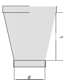
The symmetric ventilation reduction has both ends ended by connection sockets as a standard. It can also be available in other configurations, as required (socket **M** - flange **K** - spigot **B**).
